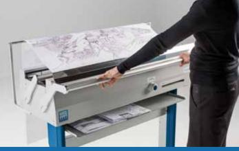
With FlexFold 1.1 fold your projects will be quick and easy! Just unlock the folding machine with the appropriate knob and open the pressure bands, put the paper and use the handle to fold perfectly at 21 cm.
