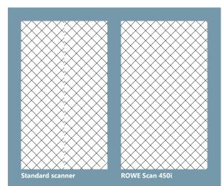
■ ROWE DYNAMIC STITCHING (RDS) (patent) ROWE engineers have achieved a groundbreaking innovation: excellent scans, even when the document is folded or thin. The patented ROWE DYNAMIC STITCHING continuously controls the scanned document data of each sensor and sets them together in real time. Any deviations that may occur are corrected automatically. Compare the difference!
